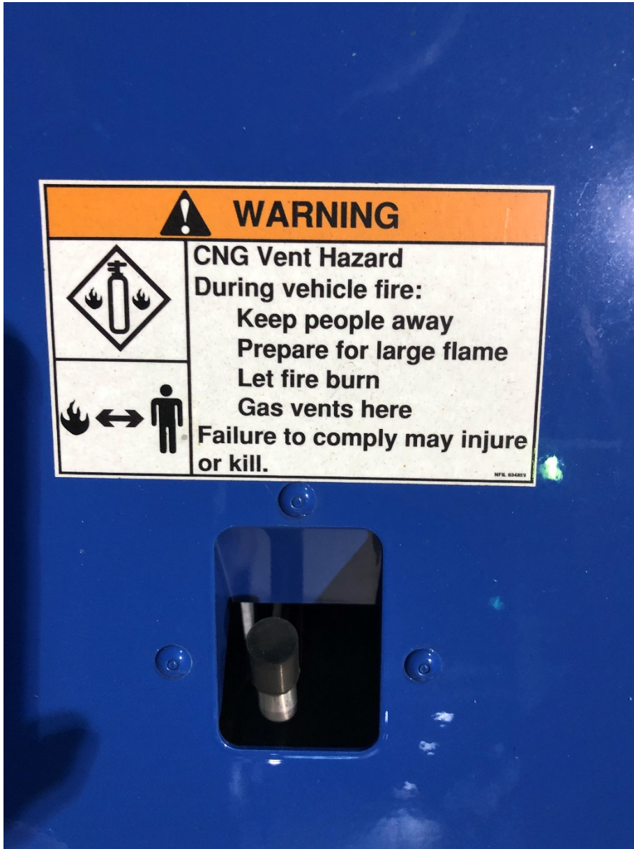
11. PRD vent line outlet (with black cap) on New Flyer CNG bus.
