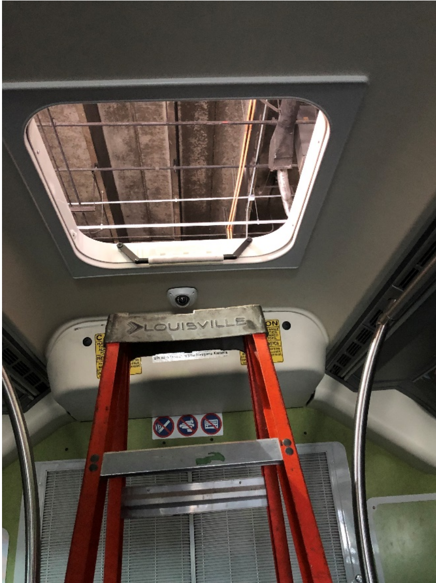
1. Access to CNG storage tank through rear roof hatch.
